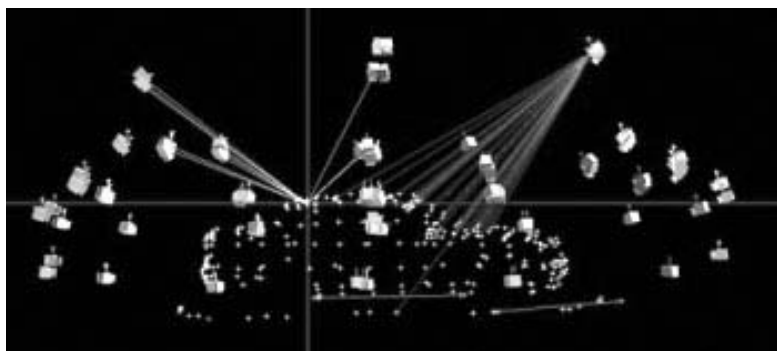
Figure 4. After the images has been taken, the software determine the camera locations, distances to each dot and measures the shape of the manufactured part.
