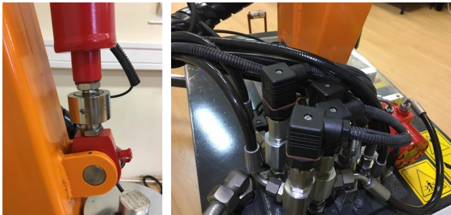
Figure 9. HBM Force sensor on lift mechanism (left) and pressure sensors (right)
