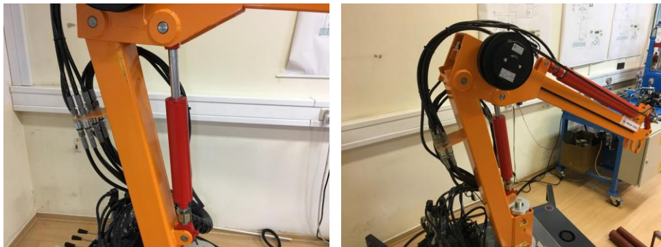
Figure 4. Double acting hydraulic cylinder for lifting of the arm by means of arm rotation
