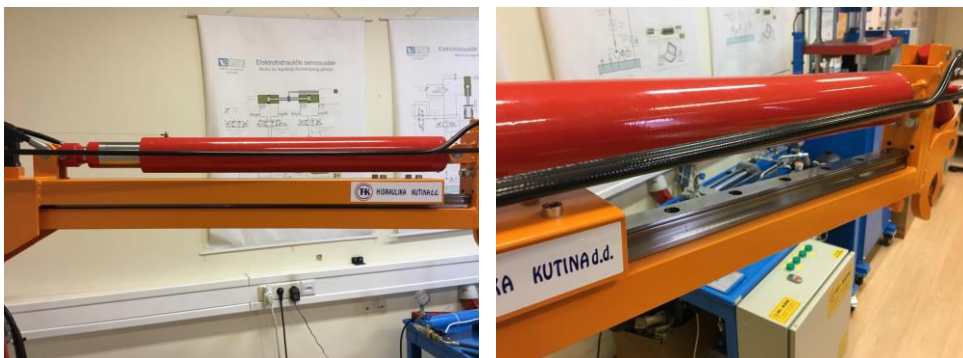
Figure 5. Telescopic double acting hydraulic cylinder for arm extension
