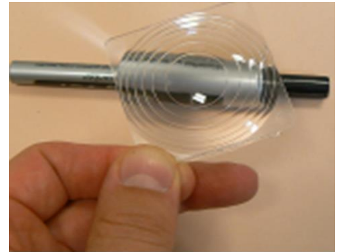
Micro-structured Fresnel lens (by injection moulding)
